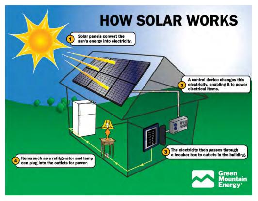
A WORKING SCHEME OF HOW SOLAR WORKS
